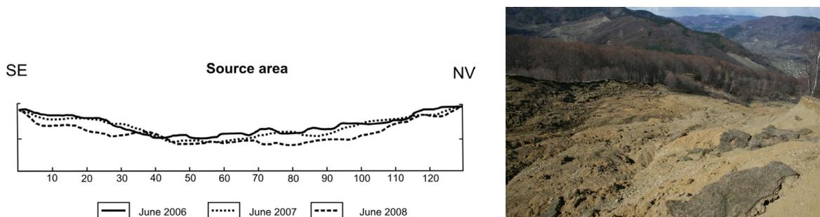
Fig. 3 – Cross-profiles in the main source area.
